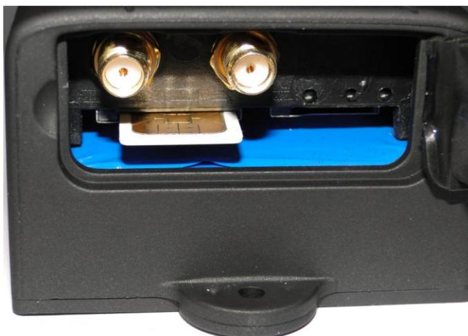
3.2 Please make sure that the SIM card is GSM network and able to execute the function of incoming calls display, no calls can be diverted and the PIN code is locked. The SMS format must be TXT format, and can't recognize the PDU format.
